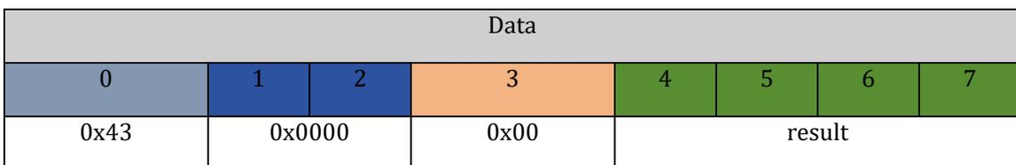
Result is the obstacle avoidance result, type INT, 0 indicates no obstacle, 1 indicates a distant obstacle, 2 indicates a near obstacle.
