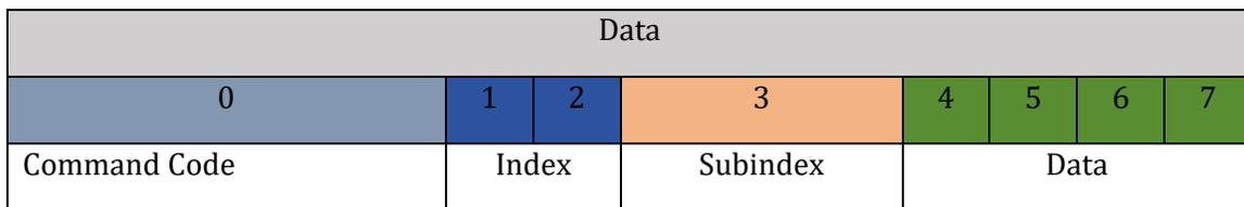
Obstacle Avoidance Module Communication Protocol: Device -> Equipment Device sends COB ID: 0x212
