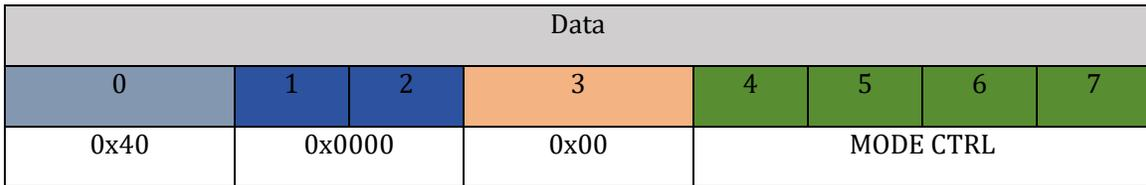
MODE CTRL is the obstacle avoidance mode, currently only 0 and 1. Equipment -> Device Device sends COB ID: 0x392
