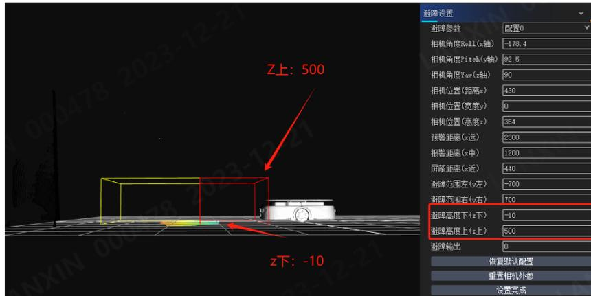
Obstacle Avoidance Output: 0 indicates no obstacle, 1 indicates an obstacle detected in the warning area (yellow box area), 2 indicates an obstacle detected in the alarm area (red box area).
